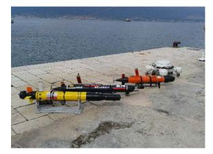
The vehicles that participated in the experiment were: a Light AUVs (Xplore1) and two X8 UAVs from the University of Porto, the Light AUV Lupis and the USV PlaDyPos from the University of Zagreb, and an IVER2 AUV from the Technical University of Cartagena. In addition, the team from University of Cyprus was responsible for making predictions used to establish the routes to be followed by these vehicles.
