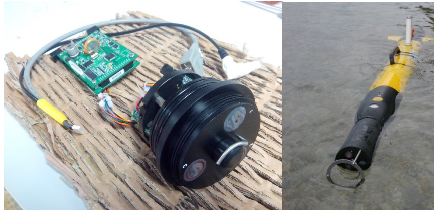
Figure 8. Left, Cyclops Integrator (Turner Designs) oil probe. Right, IVER2 Icue, with the new nose and probe integrated.
