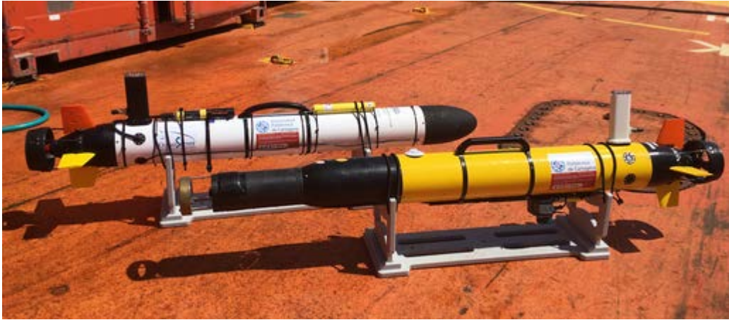
Figure 7. IVER2 with two different fluorometer integrations. White one for TUT, yellow for UPCT.
