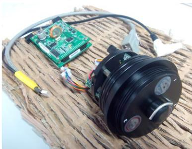
A new vehicle head has been designed by the Universidad Politécnica de Cartagena to integrate the Turner Cyclops Integrator from Turner Designs® in the IVER2 Ecomapper. A second CPU (backseat CPU) has been added to the vehicle to be in charge of recording the Oil and Rhodamine data provided by the probe and merge them with the navigation data from the vehicle.
