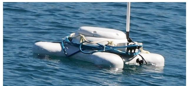
The role of this vehicle is quite important too. They are in charge of the communication between underwater AUVs and UAVs, and tracking the AUV while they are not in the surface. The vehicle used has been built and developed at UNIZG-FER for tracking of underwater objects communication router between the surface and the underwater navigation aid for the underwater.
