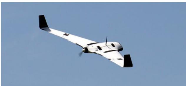
The UAVs will be used as data mules, by downloading from the AUV any data gathered during an oil spill mapping, and quickly bring it back to the nearest base station for analysis. The X8 is a low-cost COTS (Components Off-The-Shelf) vehicle, modified at the LSTS, which allows for quickly deployable surveillance missions. It's a hand launchable vehicle perfected for low altitude reconnaissance scenarios with live video feed.
